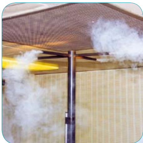
Left: Flow visualisation of moderate wind speed with no evidence of any "short circuiting" of the air movement
